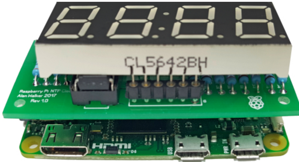
PCB Side View with 7 Segment LED attached to Raspberry Pi Zero
