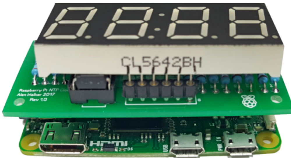
PCB with 7 Segment LED attached to Raspberry Pi Zero
