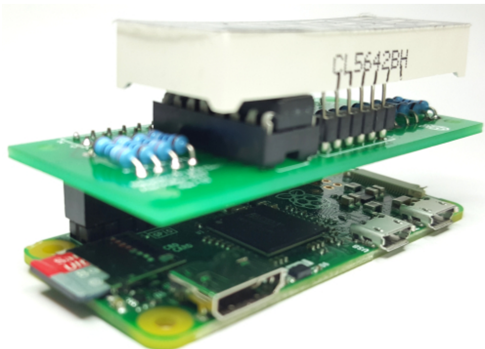
PCB Isometric View with 7 Segment LED attached to Raspberry Pi Zero
