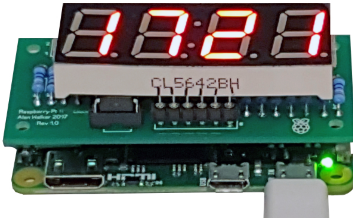
Working PCB on Raspberry Pi Zero
